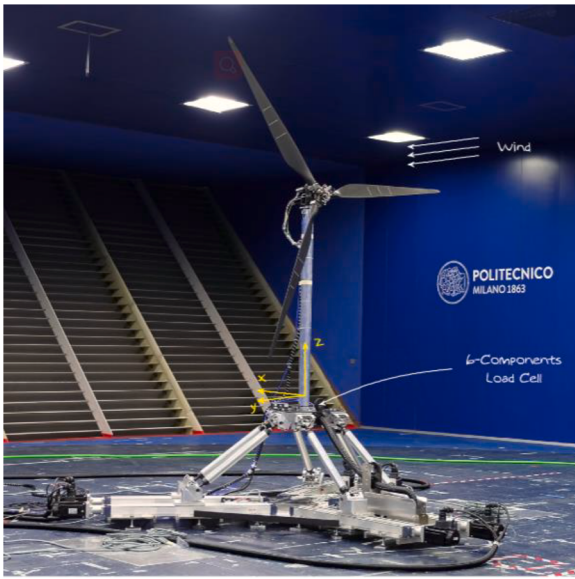
Fig. 13. Setup of the aerodynamic hybrid model test; reprinted with permission (Belloli et al., 2020).
